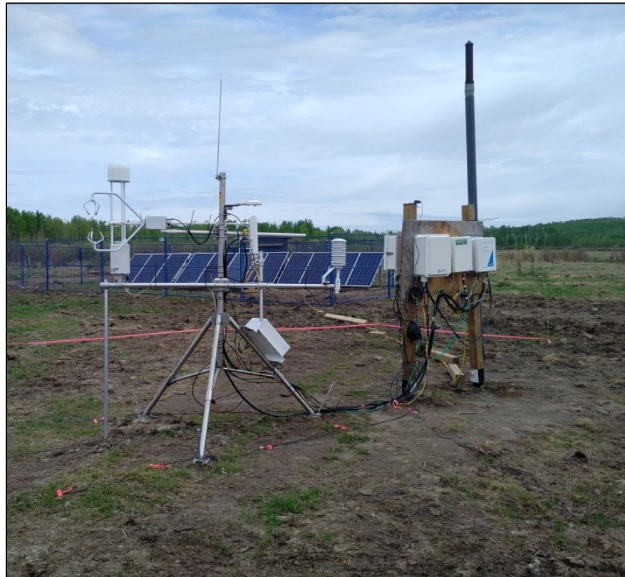
Figure 34. Hudson's Hope Field Research Station investigating natural gas migration and interactions in a shallow aquifer. Photos taken during the Panel's site visit.
