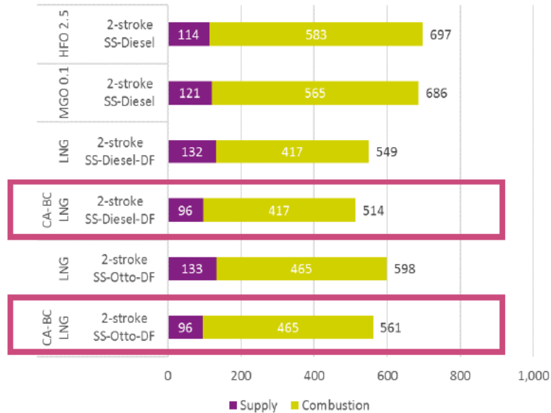
2-stroke slow speed engines: WtW - GHG IPCC -AR5 [g CO 2 -eq/kWh engine output]
